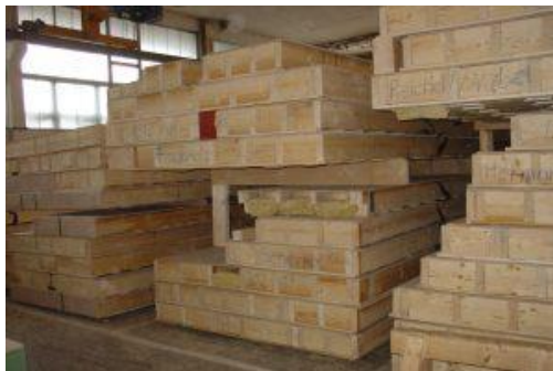
Prefabrication of house elements
